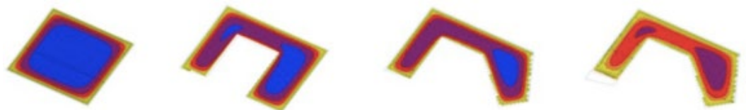
Figure 3 Depicts the Relationship Between Heat Gain and the Form of the Building Source The Edge, PLP Architecture
