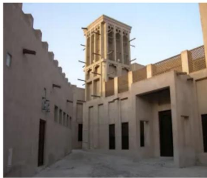
Figure 5 Barjeel Towers, Sometimes Referred to as Windcatchers or Wind Towers, are Historic Architectural Elements Engineered for Natural Ventilation and Cooling
